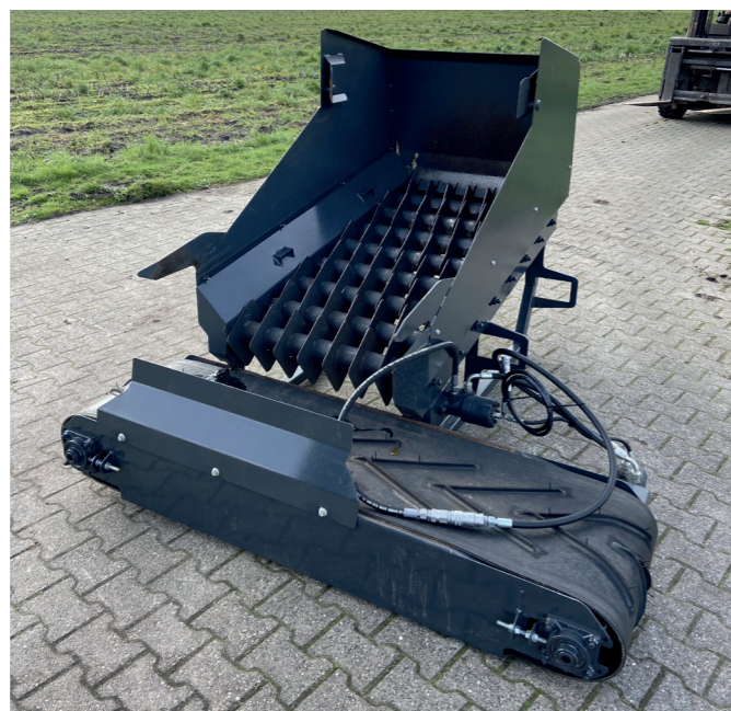
Disc screen + discharge right left under the belt
