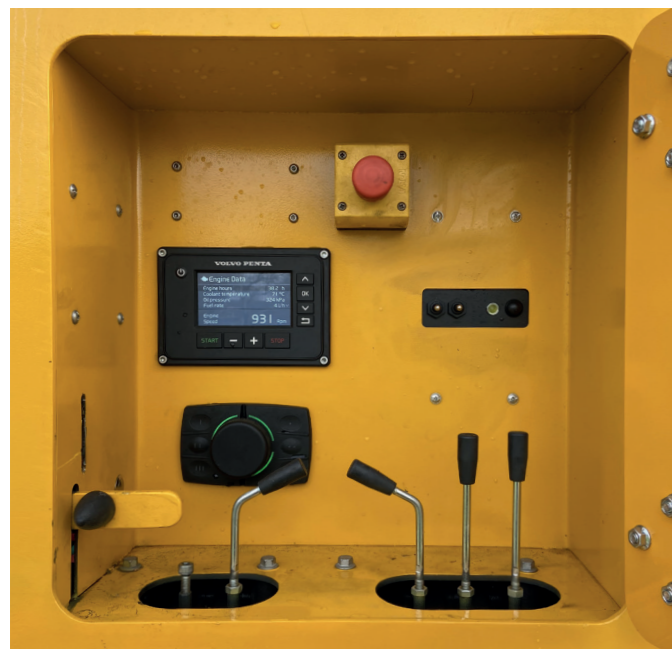
Engine controller + shredder controllers, manual override
